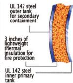
To meet UL2085 the requirement is for 3 inches or 75mm of insulation on all faces of the tank, including the roof and floor.
